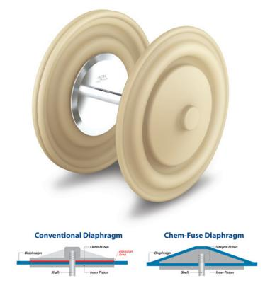
Wilden® Chem-Fuse Integral Piston Diaphragms (IPD) are designed with a piston that is integrated into the diaphragm itself. The result is that unlike conventional diaphragms, the Chem-Fuse IPD has no outer piston abrasion, which is a key failure mode for conventional diaphragms, and eliminates a potential leak point around the outer piston. This means improved diaphragm life and peace of mind when handling hazardous liquids.
