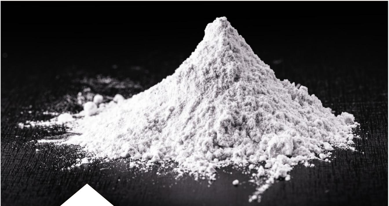
*Though titanium dioxide ( $TiO_2$ ) may appear to be a fine powder, in reality it is very abrasive in slurry form, which is its general state when used in paint and coatings production. Therefore, when AODD pumps are used in its transfer, the diaphragms must be able to withstand outer-piston abrasion, the chance of which the innovative integral piston design of the Wilden® Chem-Fuse Diaphragm eliminates.*
