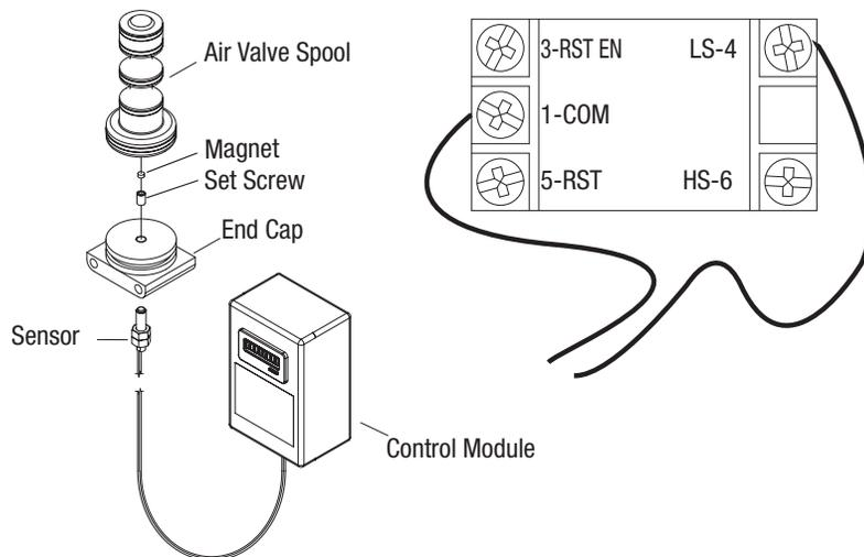
(LS) at the back of the LCD display. The wiring can be extended up to 250 feet for ease of installation.
