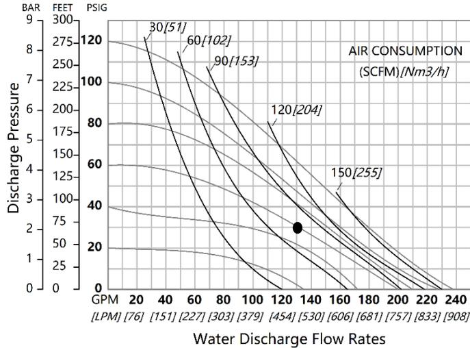
**Example:** A PR1560 metal EZ-Install Wil-Flex-fitted pump achieved a flow rate of 492 lpm (130 gpm) using 127.5Nm<sup>3</sup>/h (75 scfm) of air when run at 4.1 bar (60 psi) air inlet pressure and 2.1 bar (30 psi) discharge pressure.
