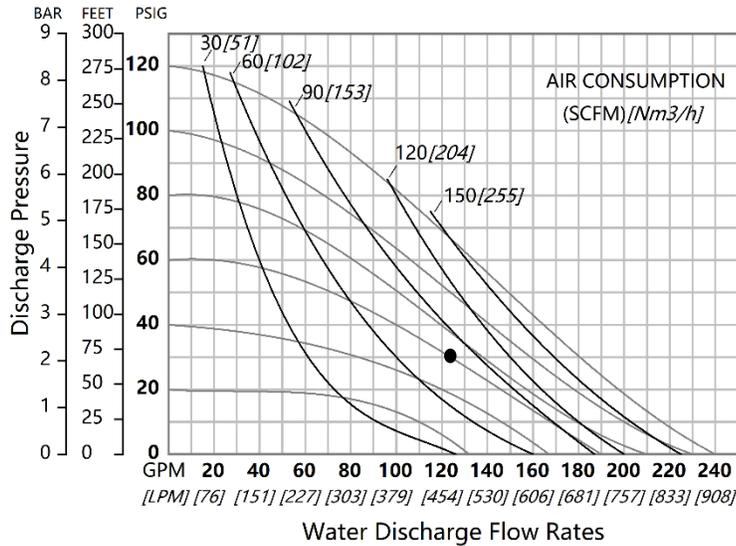
**Example:** A PR1560 metal full-stroke PTFE-fitted pump achieved a flow rate of 473 lpm (125 gpm) using 139 Nm<sup>3</sup>/h (82 scfm) of air when run at 4.1 bar (60 psi) air inlet pressure and 2.1 bar (30 psi) discharge pressure.
