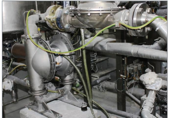
Reliability is a key characteristic of the Wilden® Advanced™ Series AODD Pumps as a single pump is required to pump base polymers to 11 different machines around the clock in Villeroy & Boch’s Wellness manufacturing operation.
