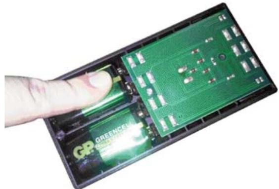
Clip back cover, checking it is correctly orientated. Put back and tight screws.
