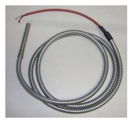
The cartridges are fitted by sliding them into the heating flanges. Heat-conducting paste shall be applied to the cartridge at the time of assembly in order to improve thermal conductivity between the flange and the cartridge. The excess of paste must be evacuated through the breather hole opposite the bore to ensure that it is not clogged. This will prevent an accumulation of humidity.
