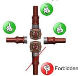
Ensure the arrow cast on the body points away from the compressor.
