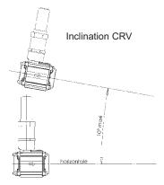
In case of the axis positioned vertically, including a flow direction going upwards, the spring **1805** (see § SPARE PARTS) has to be removed.
