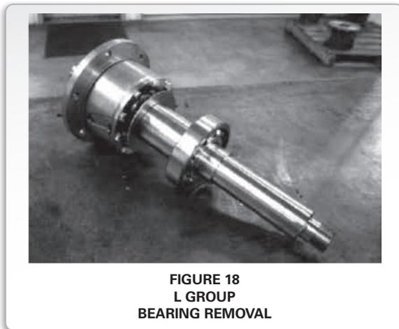
L group power ends use a clamp ring (Item 253B) instead of a snap ring to retain the thrust bearing in the bearing housing. Refer to cross-sectional view in Appendix VIII. Extract shaft/bearing housing assembly from frame as with S and M Group pump noted above.
