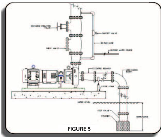
1. Suction lines when operating under lift conditions must be absolutely free from air leaks.
