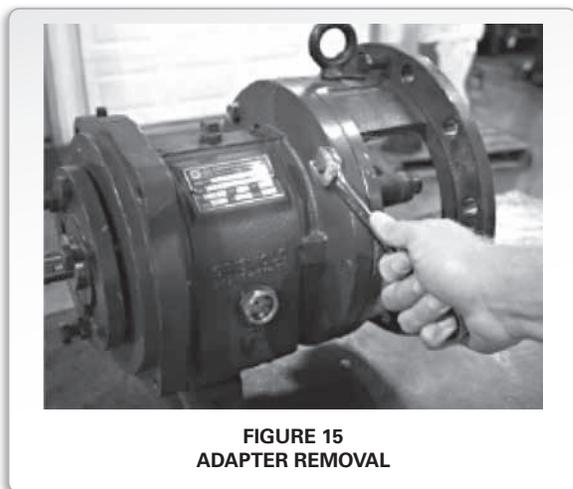
Frame adapters are used on M, L and XL group pumps. They are not used on 6" S group pumps and ring adapters are on 8" S group pumps.
