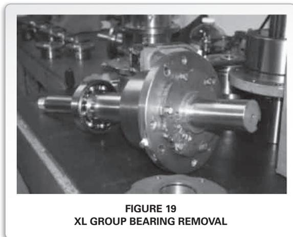
1. Remove bearing cover bolts (371C) and bearing cover (109A). Discard o-ring (Item 496). **DO NOT REMOVE LABYRINTH SEAL** (Item 332A).
