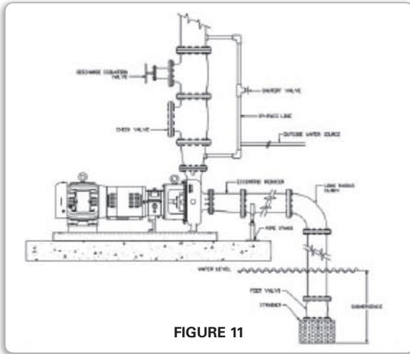
See illustration at left. Note vent location above pump discharge nozzle.
