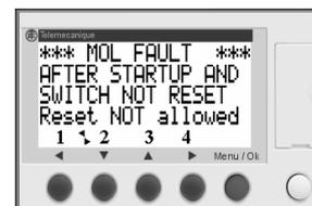
Indicates the Pumpset's current draw has exceeded the maximum allowable amperage tripping the MOL relay. It is not possible to reset the Pump Controller because the MOL relay
