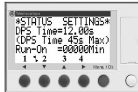
The 'Settings' screen displays the current DPS time setting (See Section 5.2.3) and the status of the 2 minute 'Run-On' feature (See Section 5.2.4).
