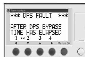
Indicates the Pumpset has not maintained the minimum required differential pressure after the DPS Time has elapsed. The Pump Controller can be reset after the reason for the
