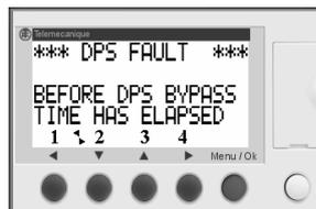
Indicates the Pumpset has not developed the minimum required differential pressure before the DPS Time has elapsed. The Pump Controller can be reset after the reason for the
