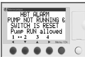
Indicates the fault as described above except the HBT switch has returned to its normally closed position. The Pump Controller will allow the Pumpset to start normally without a reset of the Pump Controller.
