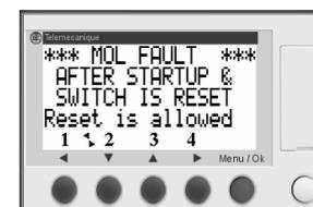
Indicates the fault as described above, except the MOL relay has automatically returned to the normally open position. The Pump Controller can be
