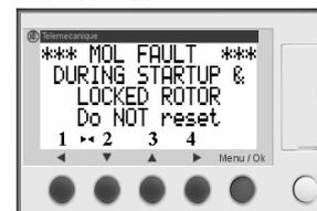
Indicates a locked rotor Motor current or short circuit condition at startup.
