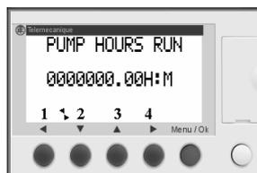
The 1<sup>st</sup> Log screen displays the Pumpset's total run hours.
