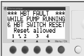
Indicates the fault as described above except the HBT switch has now returned to its normally closed position. The Pump Controller can be reset after the reason for the Fault has been evaluated and rectified.
