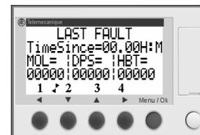
The 2<sup>nd</sup> Log screen displays the number of **specific** MOL, DPS or HBT Faults and the time (in hours and minutes) since the last Fault.
