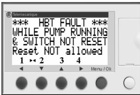
Indicates that the Pumpset's BCL™ liquid has exceeded the maximum allowable temperature while the Pumpset is running, tripping the HBT switch.
