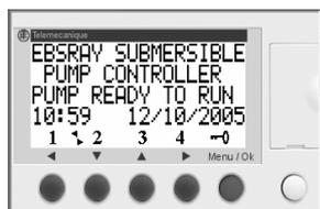
Indicates the Pumpset is idle and ready to run. The time and date are also displayed. (See Section 5.2.2 to set the time and date).
