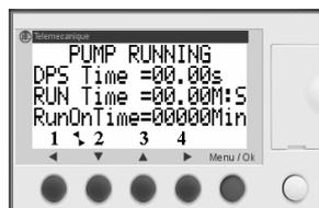
Indicates the Pumpset is running. The 2<sup>nd</sup> line displayed indicates the actual time it has taken for the Pumpset to build the minimum required differential pressure after each re-start. The
