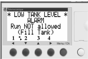
The Pump Controller has detected a low tank level via a normally open, Low Tank Level switch (if fitted). The Pump Controller will allow the Pumpset to run after the storage tank is refilled and the Low Tank Level switch opens. No other action is required.
