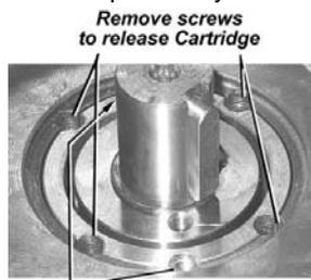
Insert screws to withdraw Cartridge
