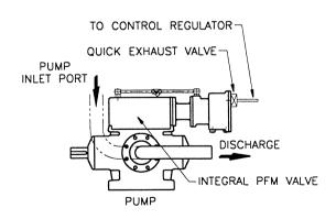
Integral Pump mounted PFM Valve Typical layout
