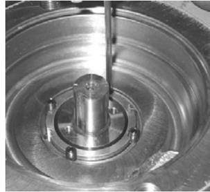
14. Lock in place with 4 setscrews (57A). Apply Loctite 243 or equivalent to setscrews
