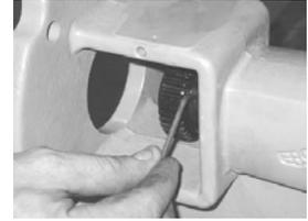
18. Check for free rotation by hand rotating the Coupling half/shaft.
