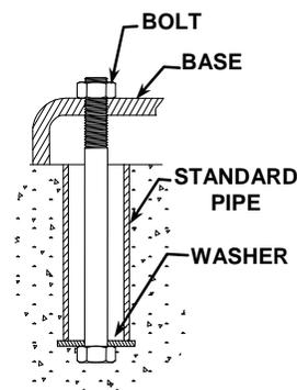
Figure 2. Foundation Anchor
