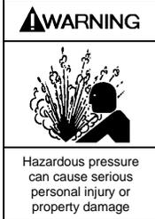
**Disconnecting fluid or pressure containment components during pump operation can cause serious personal injury or property damage.**
