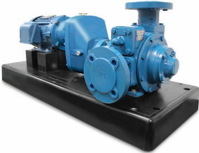
The permanently connected gearbox in the Blackmer® GNX Series Sliding Vane Pump eliminates all couplings and allows all rotating components to be totally enclosed without the need of guards, which makes it the industry's first truly alignment-free pump.
