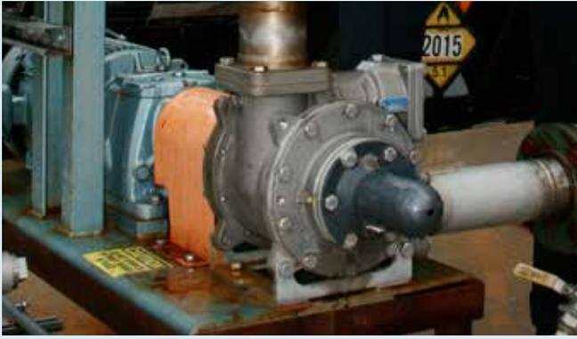
**Blackmer® SNP Series Sliding Vane Pumps offer operational advantages for two seemingly unrelated industries—the manufacture of biodiesel and soap and detergents—with waste elements from the first able to be used to create end-products for the second.**
