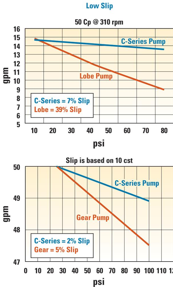
Blackmer Mouvéx C-Series Eccentric Disc pumps are capable of handling viscosities up to 10,000 Cp, working pressures to 130 psi (9 Bar), capacities of 4 to 158 gpm (15.14-598.09 lpm), operating temperatures up to 176° F (80° C), and a particle size capability range of 1-3 mm. The C-Series is also very effective at handling suspended solids with mild abrasives.
